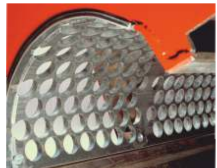
The required shredding factor for the feed material can be set using variably adjustable screens with the appropriate screen perforation.
